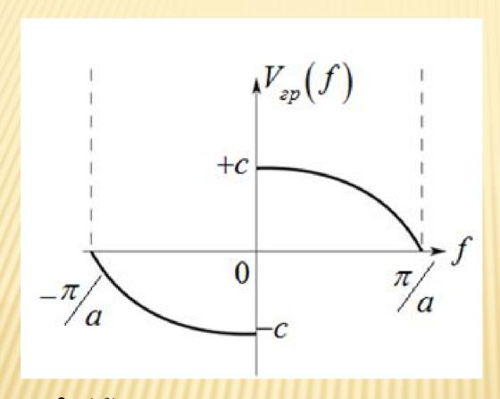
$$V_{cp}(f) = \frac{\partial \omega(f)}{\partial f}$$
